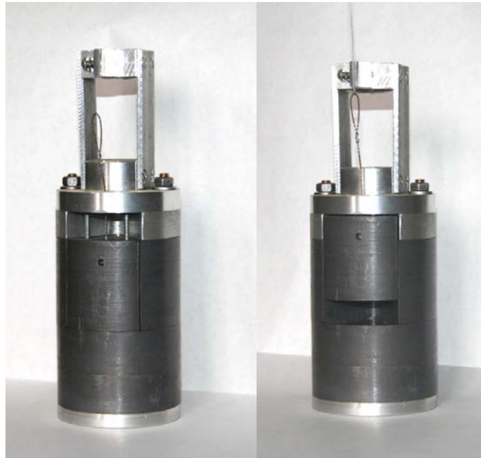
Fig.3. Collimator photos with closed lead screen (left) and open lead screen (right).
